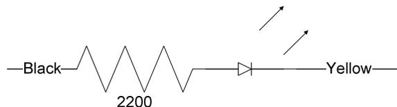
Figure 4 - LED Wiring for Second Pair
